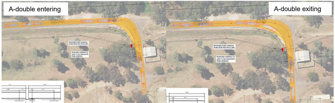
Figure 3.5 A-double entering and exiting to/from the gate
