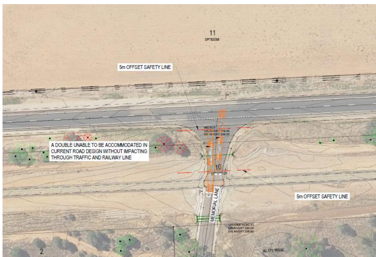
Figure 3.2 Short stacking issue with A-Doubles (existing conditions)
